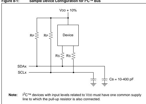
Sample Device Configuration for I<sup>2</sup>C™ Bus Figure 8-1:
